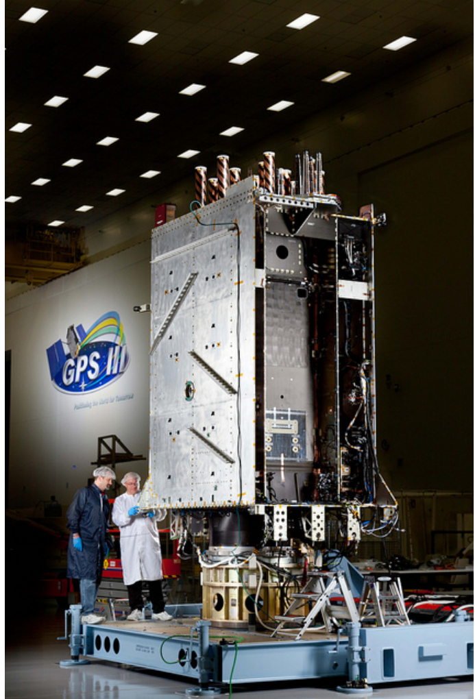
Lockheed Martin has developed GPS III with the help of the GPS Non-Flight Satellite Testbed (GNST), which serves as the program's ground pathfinder and vehicle demonstrator.
