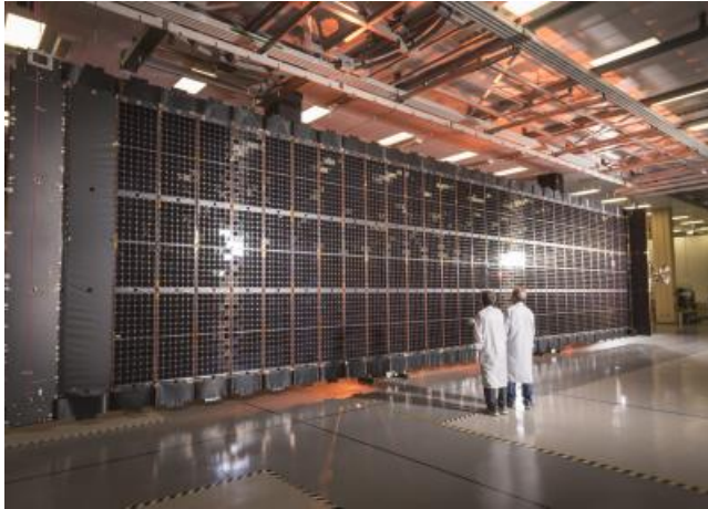
The first Multi-mission Modular Solar Array unfurls at Lockheed Martin's site in Sunnyvale, California. The reconfigurable design delivers 50 percent more power despite being 30 percent lighter.
